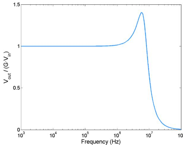
The peaking may be considered in order to avoid voltage levels that exceed the maximum ratings of the load. It can be overcome by reducing the input voltage or adding a resistor in series with the load. In some practical cases, this effect may be exploited to work at higher voltages. Please, contact us if this effect is of concern in your design.
