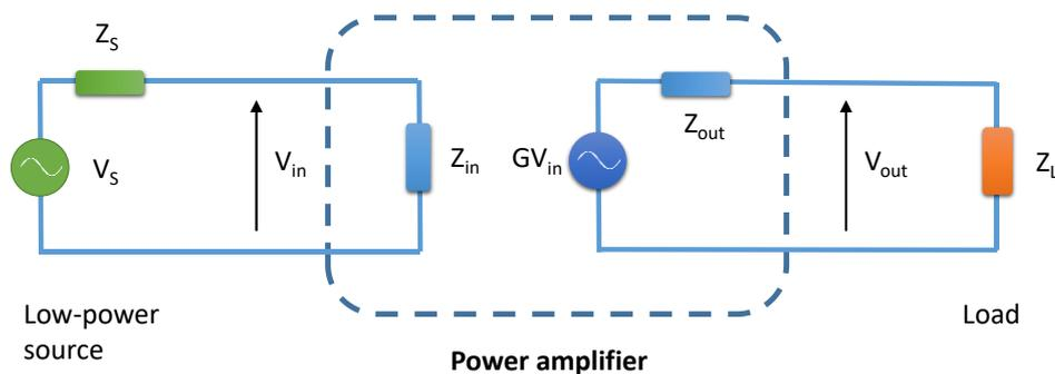
Here the input voltage  $V_{in}$  is amplified a factor  $G$  and driven to the load  $Z_L$ . However, not all this voltage is applied to the load because part of it is consumed in the output impedance  $Z_{out}$ . The actual voltage that reaches the load is:
